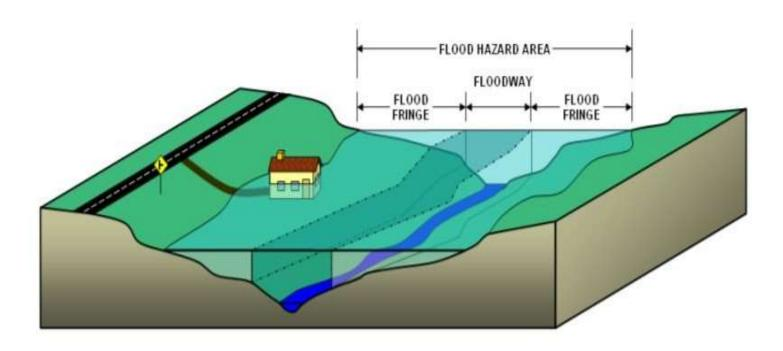
Figure 21: Flood zones (Source: NJDEP Flood Hazard Area Technical Manual)
