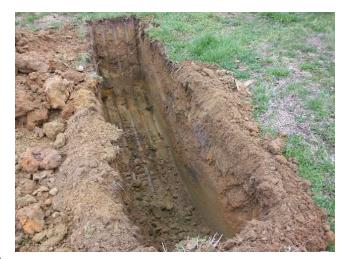
Figure 13: Test Pit Soil Profile (Source: T&M)
